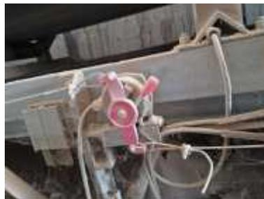
Gambar 3.10 Sensor Rope Switch
