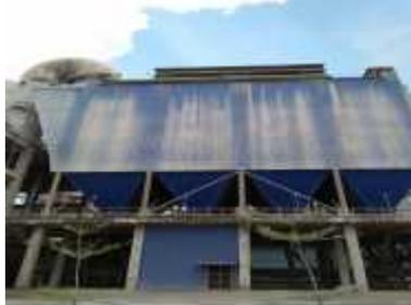
Gambar 2.6 EP (Electrostatic Presipitator)
