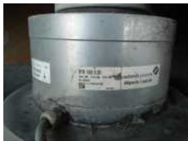
Gambar 3.11 Sensor Load Cell
