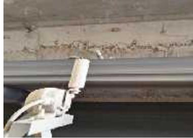
Gambar 3.9 Sensor Drift Switch
