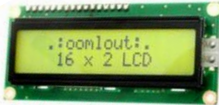
Gambar 2.4 Liquid crystal display (LCD) 16x2 [5]
