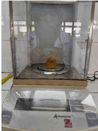
Proses penimbangan pikno + biodiesel
