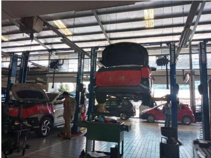
Gambar 3.7 Mengoperasikan car lift /rotary lift
