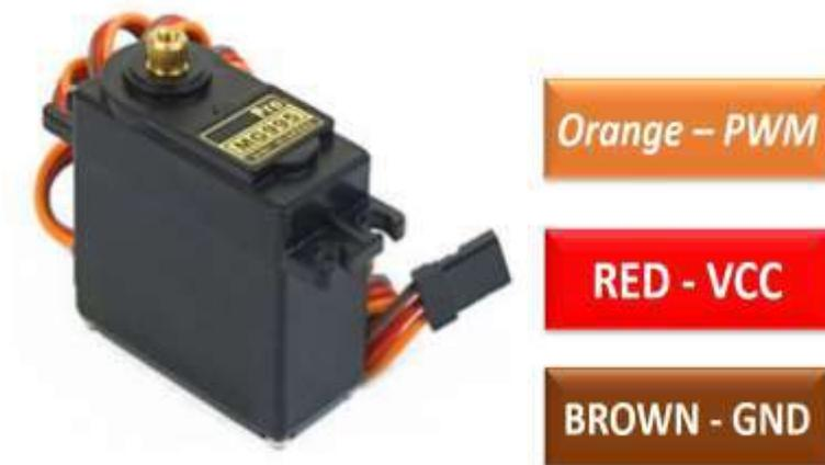
**Gambar 2.4 Motor Servo MG995**
