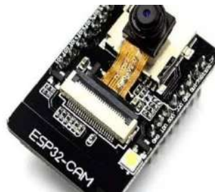
Gambar 2. 3 modul camera esp32 cam ( sumber; Febriyan Dwi hartato, 2019)
