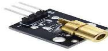
Gambar 2. 8 Sensor laser ky-008
