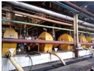
Gambar 3. 21 *Sludge Separator (Centrifuge)*
