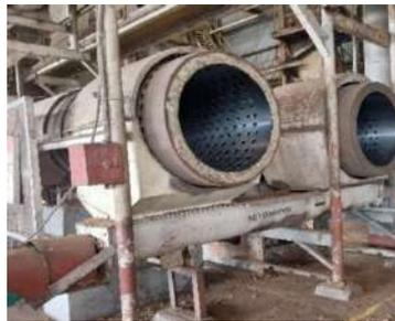
Gambar 3. 25 Nut polishing drum
