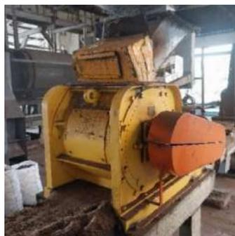
Gambar 3. 27 *Ripple mill*
