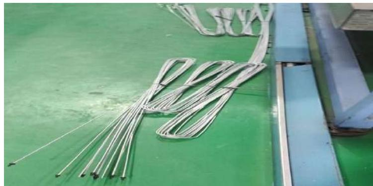
Gambar 3.3. Pipa Kondensor
