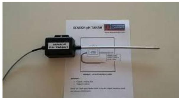
**Gambar 2.4** Sensor Ph Tanah
