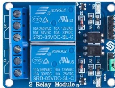
**Gambar 2.10** Modul Relay 2 Channel (Sunfounder, 2017)
